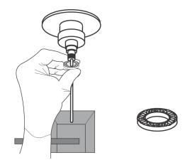
3. Install the new Bal seal spring-side up.
