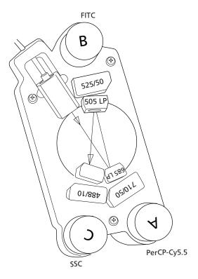
Note that with the 488-nm blue laser, FITC requires a 525/ 50 notch filter if the cytometer also uses a 532-nm laser.
