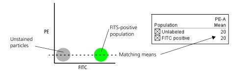
Once fluorescence compensation has been set for any sample, the compensation setting remains valid for a subsequent dim or bright sample (provided the signal is not saturated), because compensation subtracts a percentage of the fluorescence intensity. The following figure illustrates this principle. Although the signals differ in intensity, the percentage of the FITC spillover into the PE detector remains constant.
