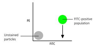
Using the **Compensation** tab of the **Cytometer** window in BD FACSDiva software, you can adjust the PE-%FITC spectral overlap value. Compensation is optimal when the positive and negative FITC populations have the same means in the PE parameter statistics.
