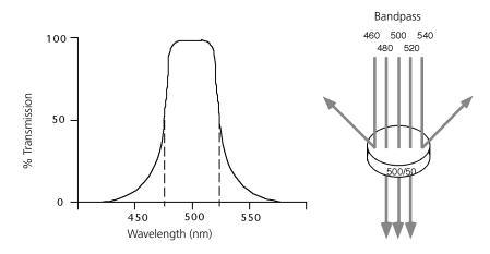
The performance of an optical BP filter depends on the optical transmission. Sample transmission curves are shown in the following figure. A filter with a narrower (steeper) transmission curve generally yields higher performance. The transmission specifications depend on the construction of the filter.
