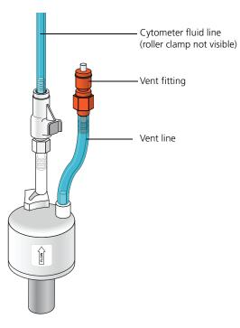
2. If bubbles are visible, gently tap the filter body with your fingers to dislodge the bubbles and force them to the top.
