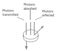
Even though an optical filter is rated at its 50% transmission point, the filter passes (lets through) a minimal amount of light outside of this indicated rating.
