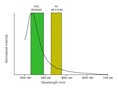
This spillover can be seen in a dot plot of FITC vs PE. The FITC spillover in the PE detector must be corrected as demonstrated in the two figures that follow.
