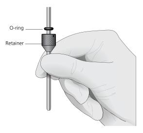
3. Invert the outer droplet sleeve and allow the O-ring to fall onto the benchtop.
