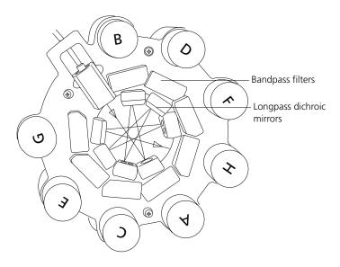
**Signal detectors** Light signals are generated as particles pass through the laser beam in a fluid stream. When these optical signals reach a detector, electrical pulses are created that are then processed by the electronics system.
