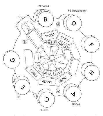
Note that when you use a PE conjugate with a 561-nm laser, you must replace the 585/42 bandpass filter (BP) with a 582/ 15 BP, regardless of which laser (blue, green, or yellow-green) is exciting the PE fluorochromes.
