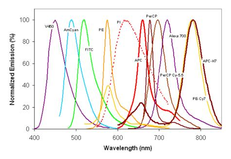
The following figure shows the emission spectra of some commonly used fluorochromes.
